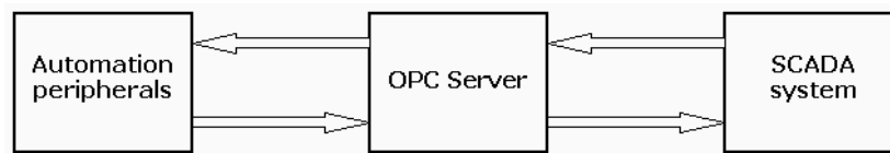
Figure 5 – Typical OPC in a SCADA System
